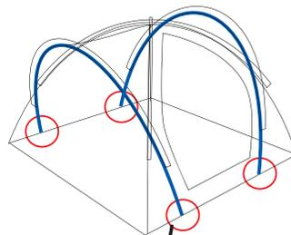
5. Peg out all the peg points around the inner tent. The peg points at the base of each pole should be pegged through the webbing loop rather than the steel ring.
