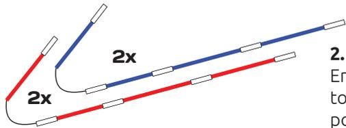
2. Assemble the 4 pole sections. Ensure that the poles do not snap together. It is important that the poles are fully inserted into the ferrules. If not connected correctly they can cause damage when tensioned.
