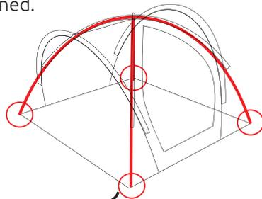
4. Thread the **BLUE** poles through the **BLUE** trimmed pole sleeves at the front and rear of the tent. Insert the pole ends into the pins located on the steel rings at the base of the tent. Attached the c-clips around the poles.
