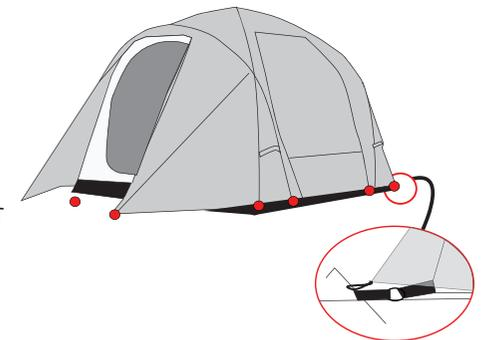
9. It is recommended that guy ropes are pegged out at all times and windows are opened whenever possible to allow adequate ventilation.
