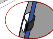
8. Attach the elastic loop over the existing inner pegs. Where there is no existing peg, peg the fly directly into the ground ensuring there is significant space between the inner and fly.
