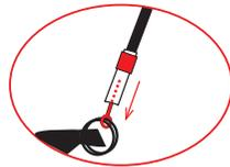
**4.** Thread the **BLUE** poles through the pole sleeves on either side of the dome you have just created. Insert the pole ends into rings. Attach the C clips around the poles.
