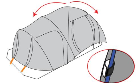
**8.** Attach the elastic loop over the existing inner pegs. Where there is no existing peg, peg the fly directly into the ground ensuring there is significant space between the inner and fly.
