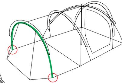
**6.** Peg out all the peg points around the inner tent. The peg points at the base of each pole should be pegged through the webbing loop rather than the ring.
