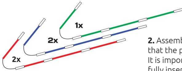
**2.** Assemble the 5 pole sections. Ensure that the poles do not snap together. It is important that the poles are fully inserted into the ferrules. If not connected correctly they can cause damage when tensioned.
