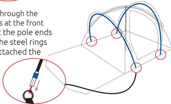
**5.** Peg out all the peg points around the inner tent. The peg points at the base of each pole should be pegged through the webbing loop rather than the steel ring. Attach the C-clips around the poles.
