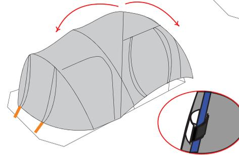
**6.** Pull the fly over the inner tent. The **ORANGE** webbing loops indicate the front of the fly.
