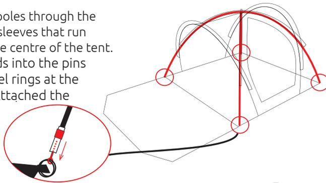
**4.** Thread the **BLUE** poles through the **BLUE** trimmed pole sleeves at the front and rear of the tent. Insert the pole ends into the pins located on the steel rings at the base of the tent. Attached the c-clips around the poles.
